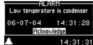
**Possible cause 1: Air in the heating system.**
