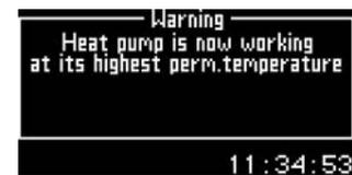
**Possible cause 3: The underfloor heating or radiator valves are closed.**
