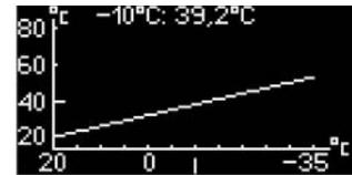
3. The most common adjustment is to increase the H value slightly to obtain more heating in cold weather. In the display you will see that the H value has been located and then marked by pressing the dial. The H value can now be changed by turning the dial. When you are happy with the H value, press the dial and select *Save*.
