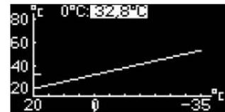
In the example to the right, the value at 0°C has been changed to 36.8°C, i.e. the flow temperature has been increased by four degrees. The dial has been pressed and *Save* has been marked. The changed curve is now saved by pressing the dial.
