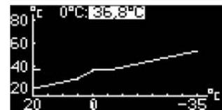
Recommended values: Increase by 4°C at outdoor temperature of 0°C and by 2°C at outdoor temperature of +5°C.
