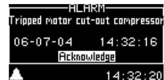
**Possible cause 2: Current level (A) on the motor cut-out is set too low. The current drawn by the compressor varies during summer/winter operations.**
