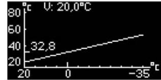
2. Start by finding the value you wish to change. It can be V, H or some other value. To find the correct value, turn the dial clockwise or anti-clockwise. At the top of the display, various outdoor temperatures with corresponding flow values on the curve are shown, at the bottom, a dash can be seen that shows the position on the outdoor temperature axis. Continue turning the dial and you will eventually find the H value. Continue turning the dial even when you see a back arrow.
