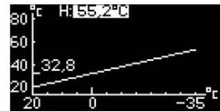
4. It may also be necessary to change a specific value on the curve, e.g. to increase the heating at temperatures around 0°C. Turn the dial to find the value at 0°C and press the dial to mark the value.
